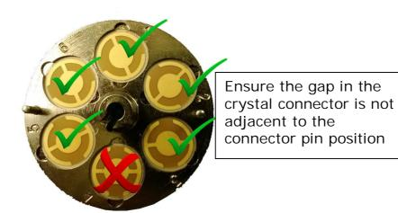
With the new crystals fitted gently snap the two halves of the crystal cassette together taking care not to break the delicate crystals. The cassette top will only fit one way on the offset pins and the stamped [0] must be on the outside of the assembly. Once the crystal cassette has been assembled we suggest it is kept horizontal to ensure the crystals do not move away from their supports.
